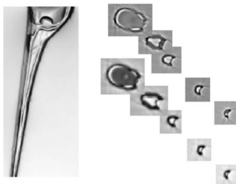
FIG. 6.12. On the left is a rendered phase-retrieved image of the bee sting used for broad-beam imaging experiments. The top diagonal series on the right are reconstructed slices through the sting obtained using the single-plane transport of intensity phase-retrieval method at 13 keV. The lower diagonal series are approximately the same slices obtained using a broad spectrum between 10 keV and 30 keV and phase retrieved using an effective energy of 16.9 keV. The propagation distance between sample and detector was 970 mm. The average diameter of the sting is \sim 100 \mu\text{m} (Figs. 5 and 6 of Peele et al. 2005, reused with permission. Copyright 2005, American Institute of Physics).
