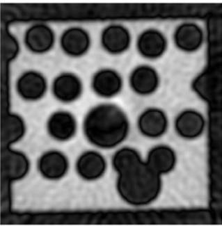
FIG. 15.11. Aluminium block with different holes, diameter = 2, 3 and 4 mm. Reconstruction with integrated data. Taken with permission from Strobl et al. (2004a).
