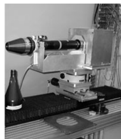
FIG. 10.6. Inline detector using reflective optics. Courtesy: ESRF, Instrument Support Group.
